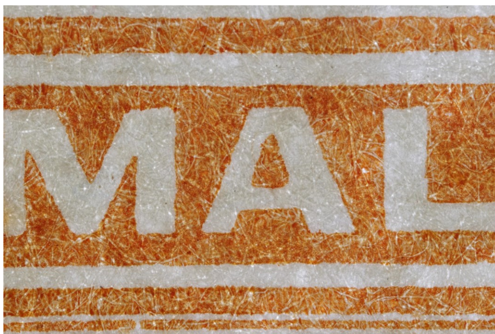
Figure 2. Close-up of striated paper under transmitted light, showing randomly oriented fibres.
